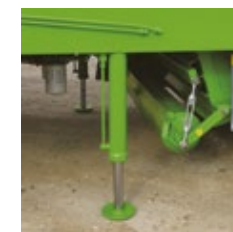
Hydraulic feet bracket and rear ladder roller
