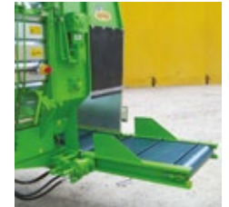
Conveyor belt extension
