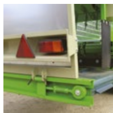
Conveyor belt with control tension device
