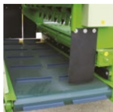
Conveyor belt width: 750 mm Side conveyor belt
