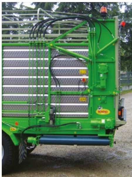
LATERAL UNLOADING BY PROPER DOSING WITH RUBBER BELT L=1400 mm HYDRAULICALLY RETRACTABLE
