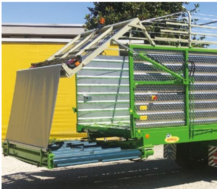
LATERAL UNLOADING CONVEYOR L=1400 mm HYDRAULICALLY RETRACTABLE
